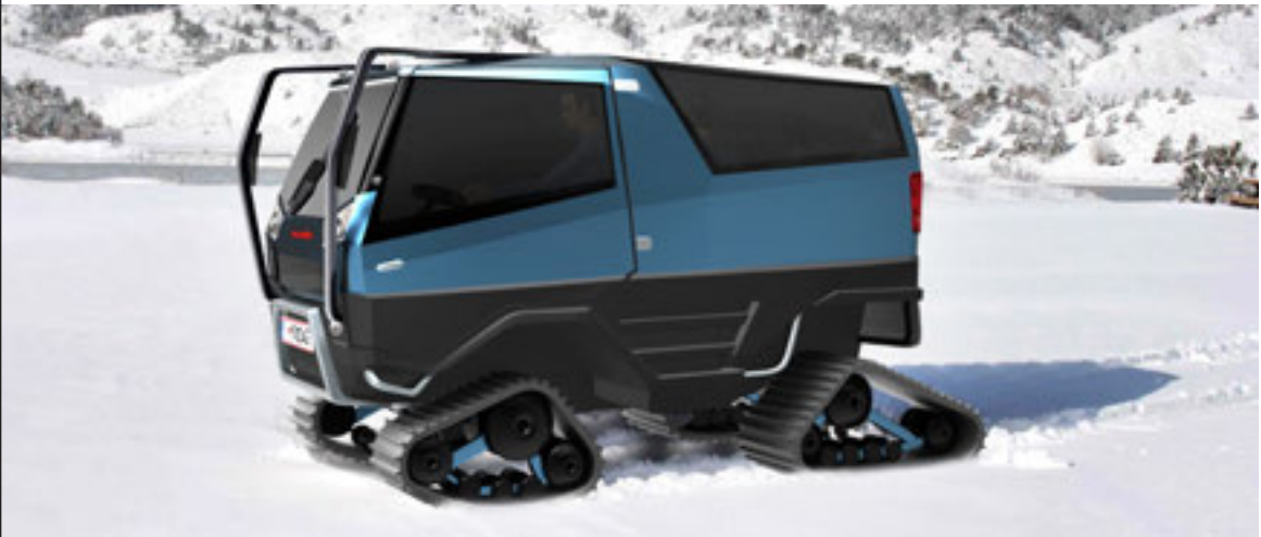
The rendering shows A-pillars and rear mirrors, the driver's door with stirrups and the all-terrain chain drive.
